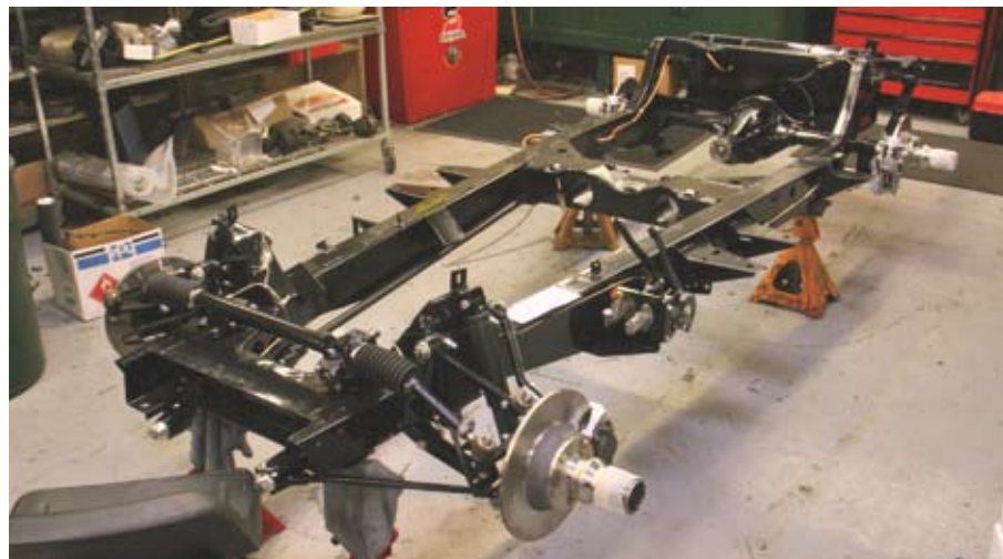
Original steel-girder frame, rivaling London Bridge for stoutness and longevity, gets fresh underpinnings such as lightweight control arms, disc-brake and rack-and-pinion conversions.
