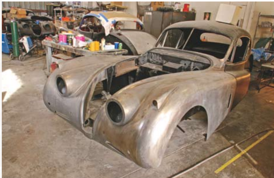
At XKs Unlimited, bodywork restoration tasks take place in a dedicated shop complex. One early XK fixed-head coupe gets its new metal massaged in the foreground.
