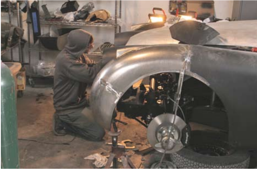
Any Jaguar needs proper ministrations. Hand-formed fenders are laboriously shaped and welded for this fixed-head-coupe XK. The upgrade to beefy disc brakes with Wilwood calipers gets a nod, too.
